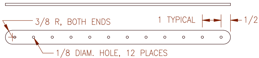
SKID PLATE, 3/4 X 1/8 ALUM. BAR, 12 IN. LONG
